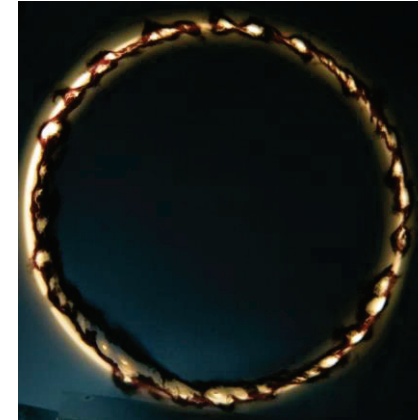
Beam imprints on thermal paper a) at the anode plate, b) backside illumination of the slit with imprint of the beam.
