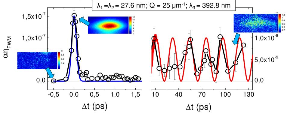
$\Delta t \approx 0$ : sharp TG peak (R<sub>cc</sub>( $\Delta t$ );  $\approx 130\text{-}140$  fs FWHM, resolution limited)  $\rightarrow$  electronic response (coherent spike) TG signal extends up to  $\Delta t \approx 100$  ps  $\rightarrow$  Longitudinal acoustic mode at (almost) the expected frequency ( $\omega_{LA} = c_sQ \approx 0.145$
