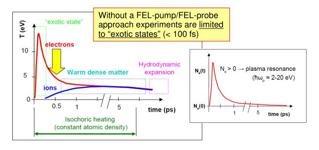
$\omega < \omega_p$ : high reflectivity and limited penetration depth (large <u>excitation</u> <u>gradient</u>)
