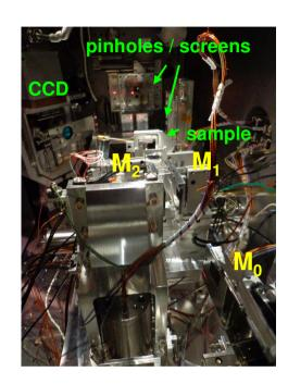
Alignement (reference pinholes + screens)  $\rightarrow \delta\theta \approx 0.2^{\circ}$ Degrees of freedom: M<sub>1,2,3</sub> pitch-roll-Z-Y; M<sub>1,2</sub> X; sample/sample pinhole X,Y,Z,pitch,roll
