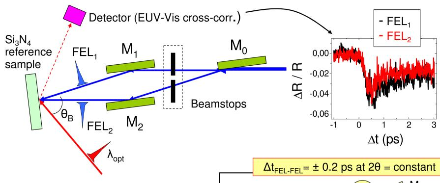
If TR signals are equal, then all pulses are in time-space coincidence and similar FEL fluence in the interaction region
