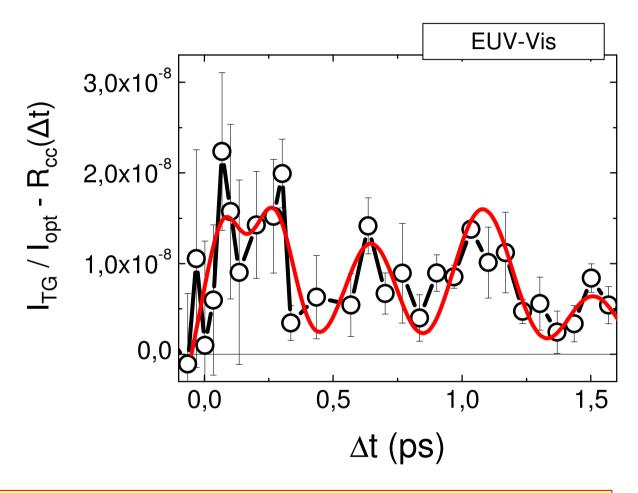
$\Delta t = 0-1.5 \text{ ps: } \text{two oscillations} \text{ ("optic modes") at } \omega_1 \approx 7.2 \text{ THz (F}_1 \text{ hyper-Raman mode } \rightarrow \text{ tetrahedral rotations) and } \omega_1 \approx 26 \text{ THz (v}_{2b} \text{ Raman mode } \rightarrow \text{ tetrahedral bendings)}.$
