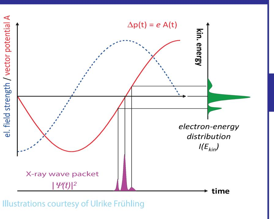
By measuring the spectrum of the electrons by Electron Time-of-Flight Spectrometers (eTOFs), one can extract the arrival time of the
