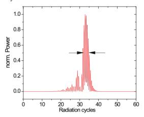
Figure 3: The seed spike's FWHM is around 3-4 radiation cycles.
