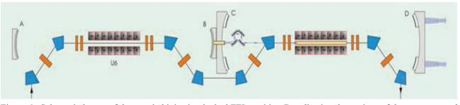
Figure 6: Schematic layout of the coupled injection-locked FEL cavities. By adjusting the settings of the resonator and the undulator modules in the respective cavities (basically cavity loss and slippage) the contribution arising from the injection locked FEL to the circulating power in the amplifier cavity can be varied. Note that the shown components are not scaled.
