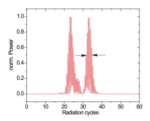
Figure 5: Double spike generation at saturation. The delay between the pulses amounts to  $\sim 200$  fs.
