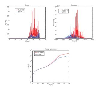
Figure 7: Power profile (top left) and spectrum (top right) at the end of the beamline and the energy gain curve (bottom). Results with the RWW on (off) are shown in blue (red).
