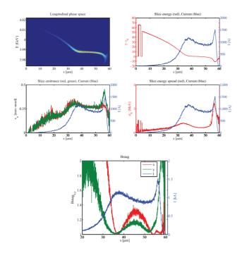
Figure 1: Longitudinal phase space (top left), slice energy (top right), x (green) and y (red) slice nomalized emittance (middle left), slice energy spread (middle right), and matching parameter (bottom) for the 100 pC S2E electron beam. The blue curves are the current and assist in locating the slice properties within the electron beam longitudinal profile.
