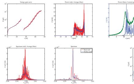
Figure 6: The energy gain curve (top left), power profile (top right) and spectrum (bottom left) for 10 independent runs (red) and their average (blue) using the 100 pC S2E electron beam. The bottom right figure shows the spectrum resulting from the amplification of a perfect seed (blue) and the real seed coming from the monochromator in the second state of the SXRSS beamline.
