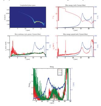
Figure 2: Longitudinal phase space (top left), slice energy (top right), x (green) and y (red) slice normalized emittance (middle left), slice energy spread (middle right), and matching parameter (bottom) for the 20 pC S2E electron beam. The blue curves are the current and assist in locating the slice properties within the electron beam longitudinal profile.
