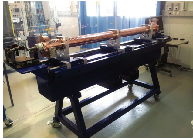
Figure 4: Transport girder for the transfer of structures from the brazing area on the PSI campus to the external storage area.
