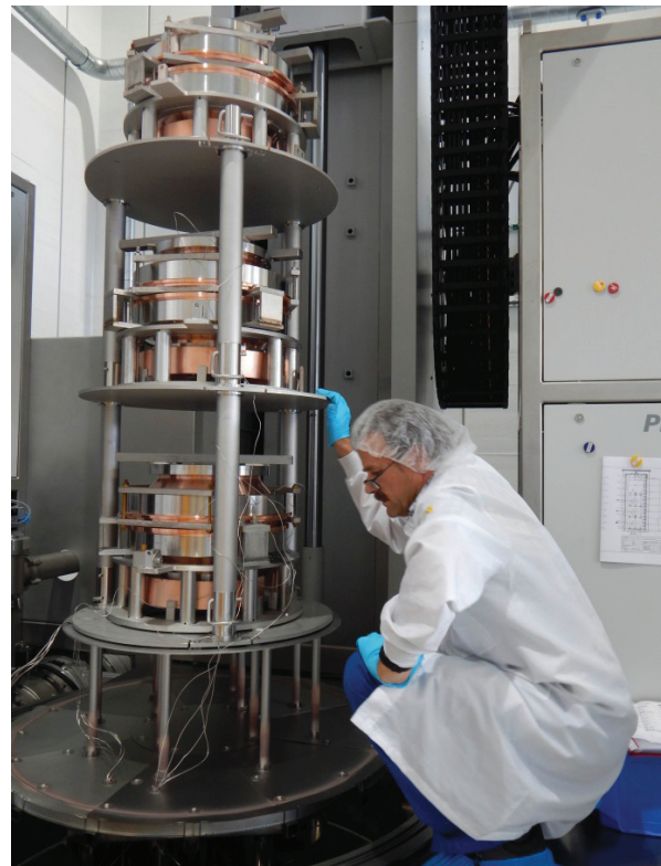
Figure 5: For the first brazing at 850°C three BOC pulse compressors in their solder gauges are arranged in a frame (total weight 640 kg) which is on a stationary table.
