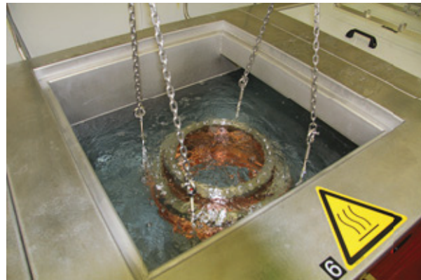
Figure 4: Ultrasonic cleaning of a BOC pulse compressor in one of the aqueous chemical liquids.
