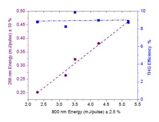
Figure 2: Measured third harmonic pulse energy (left axis,  $\bullet$ ) and conversion efficiency (right axis,  $\bullet$ ) as a function of fundamental pulse energy. Due to generation of non-linear effects the fundamental beam energy is kept below 5 mJ/pulse.
