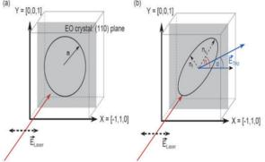
Figure 1: Refractive index ellipsoid of ZnTe Electro Optic crystal (a) Symmetric ellipsoid, without electric field and (b) The directions and the magnitudes of the main axes are changed, when an electric field is applied.
