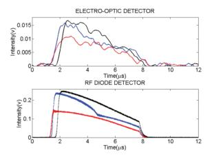
Figure 3: Experimental results for measuring the pulsed beam radiation using the EO crystal ZnTe (top graph) using the configuration of Fig. 2.for comparison the same pulses were measured simultaneously using an RF diode.
