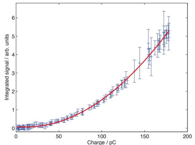
Figure 5: A plot of integrated diffraction radiation as a function of bunch charge shows a quadratic dependency. This measurement was performed without using the bunch compressor. Blue: data, red: quadratic fit.
