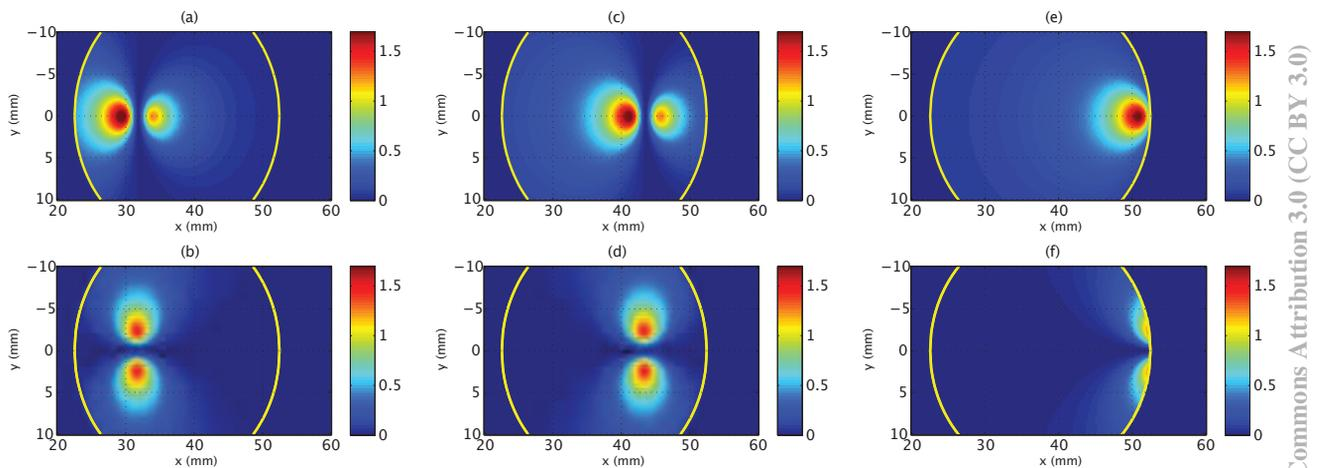
Figure 2: Radiation intensity distribution in arbitrary units on the vacuum window as a function of bunch compressor angle. The wavelength used is 2.85 mm. (a) Horizontal polarization, 3 degrees, (b) vertical polarization, 3 degrees. (c) and (d) 4.1 degrees. (e) and (f) 5 degrees.
