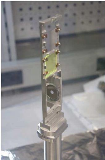
Figure 4: The diffraction radiation foil consists of a  $1\ \mu\text{m}$  thick titanium foil that has a round hole with 3 mm radius. It is placed on the same mount as a scintillating screen and an OTR target for a screen monitor.
