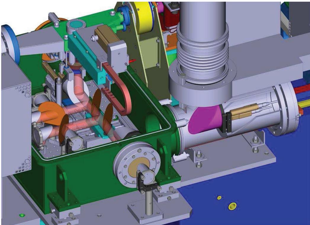
Figure 3: Technical drawing of the planned CSR bunching monitor. The fourth dipole magnet of the bunch compressor can be seen on the left. Four pyroelectric detectors are installed in an evacuated box (shown in green). The transfer line to the Martin Puplett interferometer on the tunnel roof is shown on the right.
