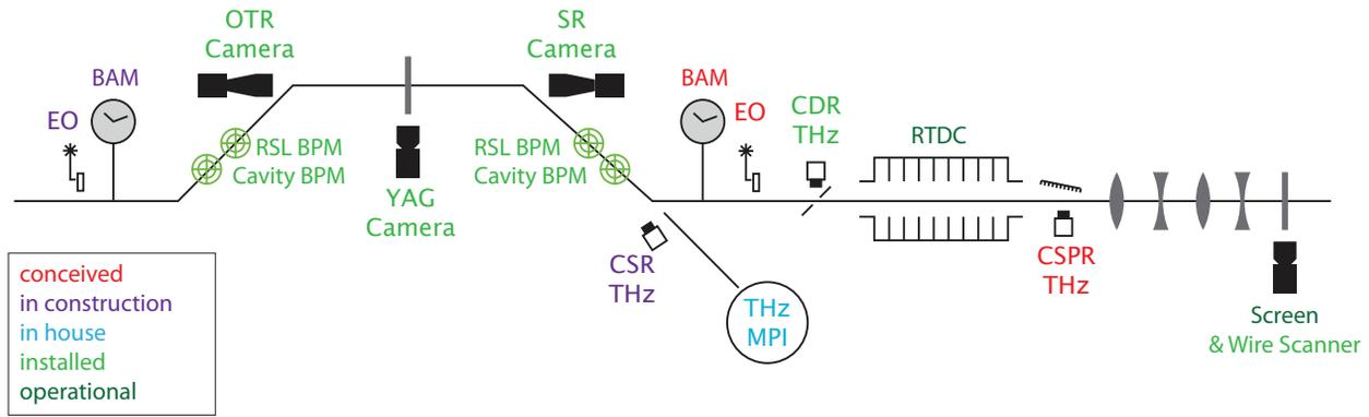
Figure 1: Instrumentation around the bunch compressor in the SwissFEL Injector Test Facility. BAM: Bunch Arrival Monitor, BPM: Beam Position Monitor, CDR: Coherent Diffraction Radiation, CSRP: Coherent Smith-Purcell Radiation, CSR: Coherent Synchrotron Radiation, EOM: Electro-Optical Monitor, MPI: Martin Puplett Interferometer, OTR: Optical Transition Radiation, RSL: Resonant Stripline, RTDC: RF Transverse Deflecting Cavity, YAG: Yttrium Aluminum Garnet.
