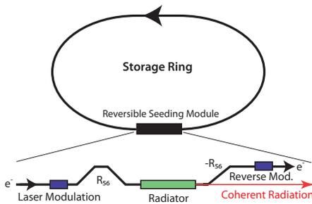
Figure 1: Schematic of the reversible HGHG scheme. A modulation and dispersive region produce microbunching according to the HGHG process. A radiator then extracts coherent radiation at a high harmonic of the seed wavelength, before an opposite sign dispersive region and second modulation reverse the HGHG process and return the beam to its original state.
