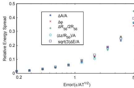
Figure 2: Equilibrium energy spread as a function of manipulation and beam errors. Simulations track each point for several damping periods to reach steady state. Parameters are given in Table 1, with the exception of harmonic number,  $H = 10$ , so that we can ignore the  $E_0$  term and use Eq. 5. We find that when relative errors are larger than the dimensionless parameter  $\epsilon/A$ , the energy spread increases significantly, confirming Eqs.7 and 9.
