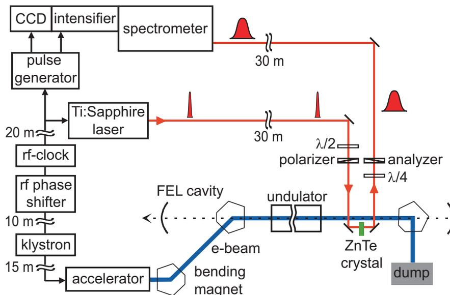
Figure 2: (color) Experimental setup at the FELIX facility. The spectrum of the Coulomb field of a single bunch is measured inside the FEL cavity at the exit of the undulator. The laser system and the spectrometer are located outside the accelerator hall. See text for details.
