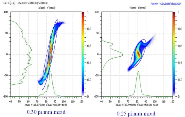
Figure 8: Argon 12+ emittance at 45 kV.
