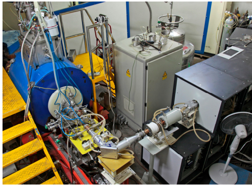
Figure 1: SECRAL with 24GHz/7kW gyrotron system.
