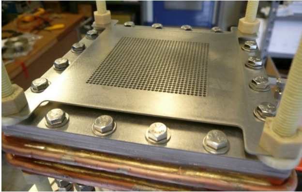
Figure 7: COMIC-array low energy with grid extractor (gap size : 4 mm)
