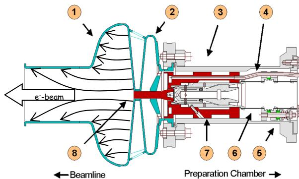
Cavity: Niobium ½ cell, TESLA 1.3 GHz
