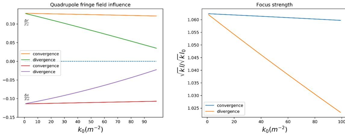
Figure 4: Quadrupole fringe field effects. In left figure  $\frac{\delta l}{l_0} = \frac{l_f - l_0}{l_0}$  or  $\frac{l_d - l_0}{l_0}$  and  $\frac{\delta k}{k_0} = \frac{k_f - k_0}{k_0}$  or  $\frac{k_d - k_0}{k_0}$ .
