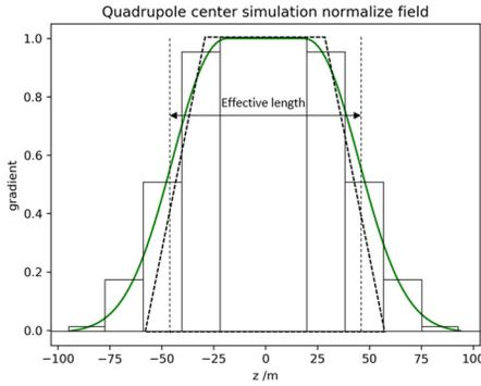
Figure 2: Quadrupole center magnetic field gradient
