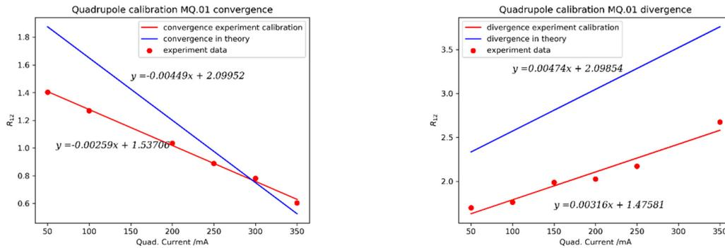
Figure 5: Quadrupole focus and defocus strength calibration.
