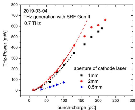
Figure 4: Measured THz power vs. bunch charge.
