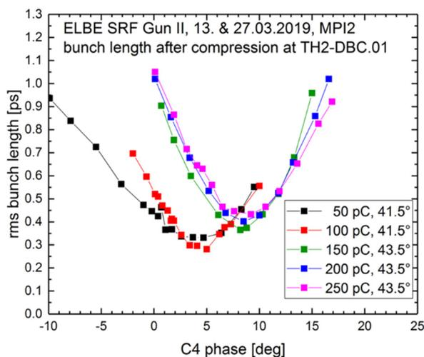
Figure 3: Bunch length measurement after compression with Martin-Puplett Interferometer (MPI). The optimized bunch length is about 300 fs.
