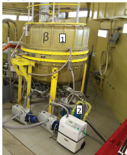
Figure 1: Accelerator BETA-8: 1 – accelerating cavity; 2 – exhaust cart.
