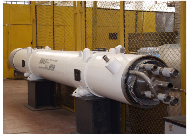
Figure 1: UNK SC dipole magnet.
