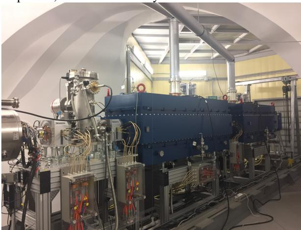
Figure 3: Interdigital H-type cavities IH1 and IH2 at JINR
