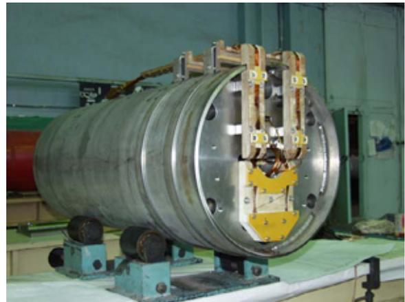
Figure 2: SIS300 high field fast cycling dipole model.
