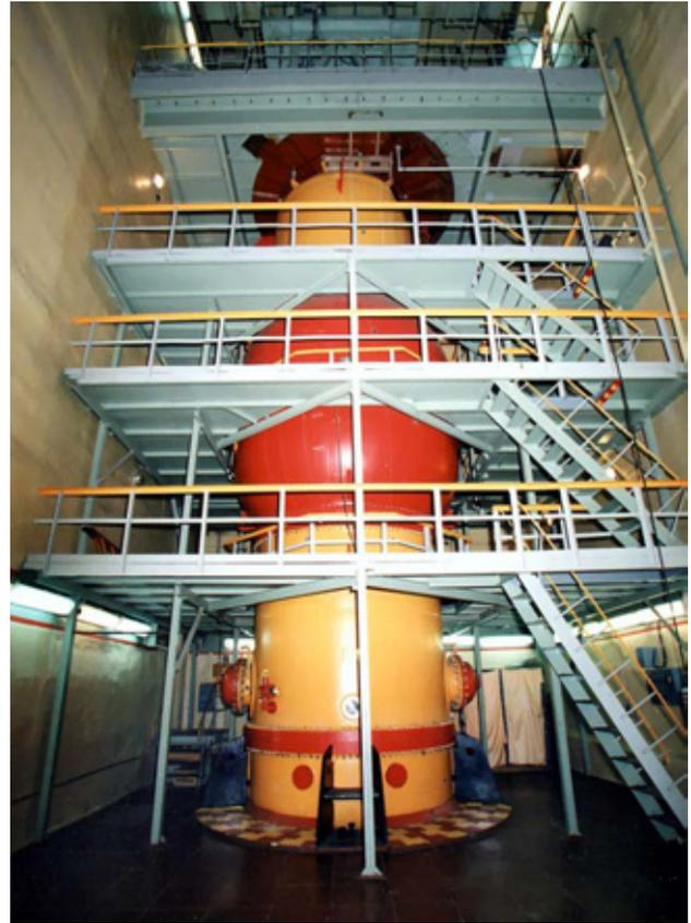
Figure 1: The EGP-15 tandem electrostatic accelerator.
