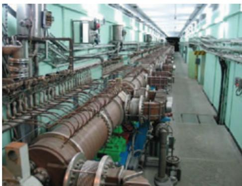
Figure 1: DAW accelerating structure in the INR linac.
