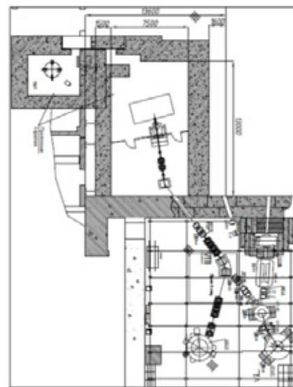
Figure 2: Scheme of synchrocyclotron with beam delivery channel and modernized medical cabin in demonstration center of proton therapy.
