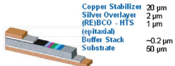
Figure 3: Structure of 2-G HTS tape (Re)BCO.
