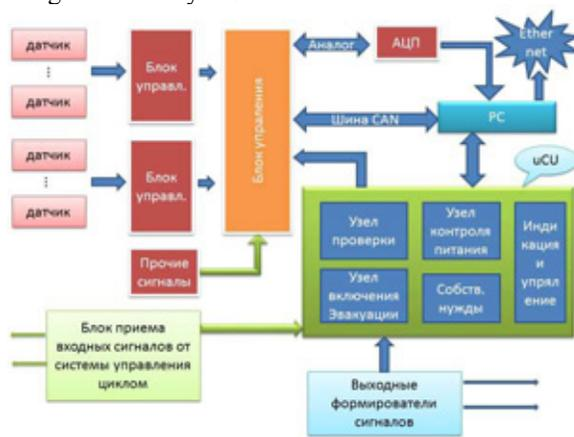
Figure 1: Block-diagram of the Nuclotron quench detection system.
