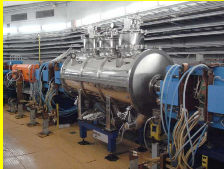
SC wiggler installed in dispersion-free straight section of SIBERIA-2
