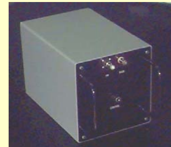
Beam Loss Monitor (Neutrons) for SNS Linac
