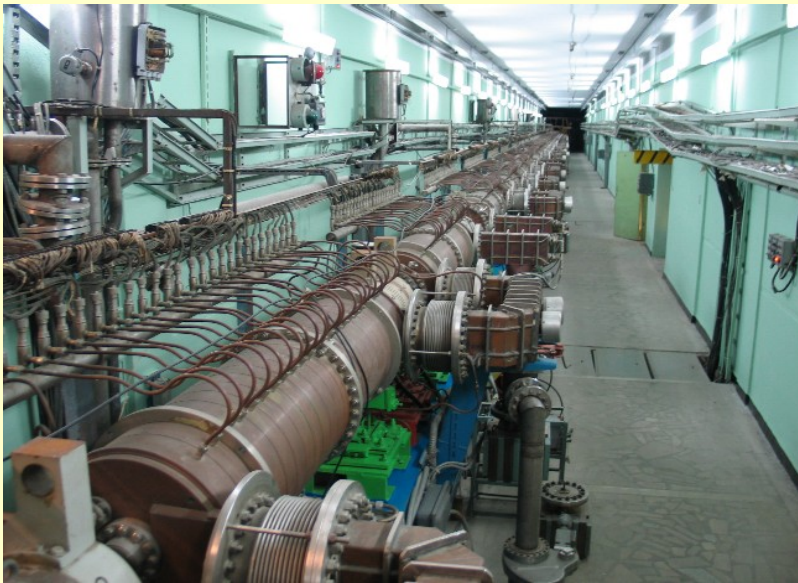
Accelerating cavities of high energy part of accelerator
