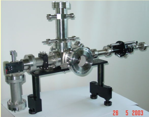
BSM developed for SNS Linac
