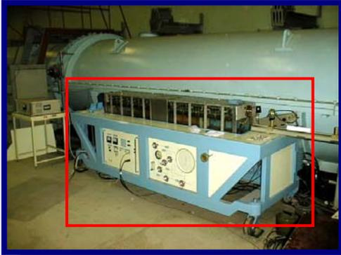
IHEP laser (CO<sub>2</sub>, 2.7 J, 10 μm, 0.25 Hz)
