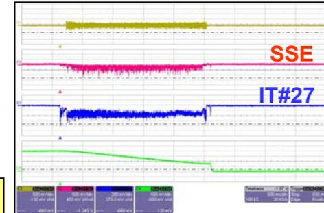
Extraction of 63% in 2.9 s.  $\sigma = 0.40$ , duty factor  $\langle \Phi \rangle^2 / \langle \Phi^2 \rangle = 0.87$ . No lines of mains harmonics
