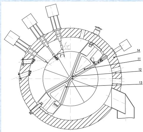
**1-electromagnet; 2- stripping unit; 3- stripping unit; 4- probe; 5- RF power bushing; 6-RF probe; 7- AFT trimmer; 8- external injection system; 9-gate valve; 10- cryopump; 11- resonance system; 13-puller; 14- vacuum chamber**
