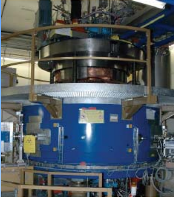
New PSI superconducting cyclotron at 250 MeV
