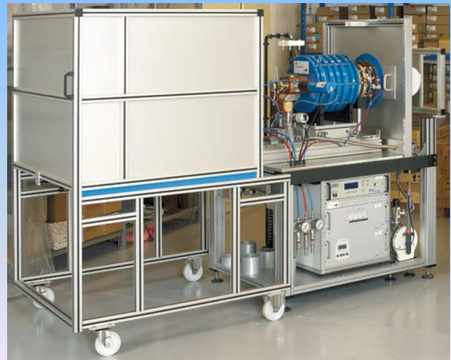
C 6+ carbon ion source, I=3 \mu A
