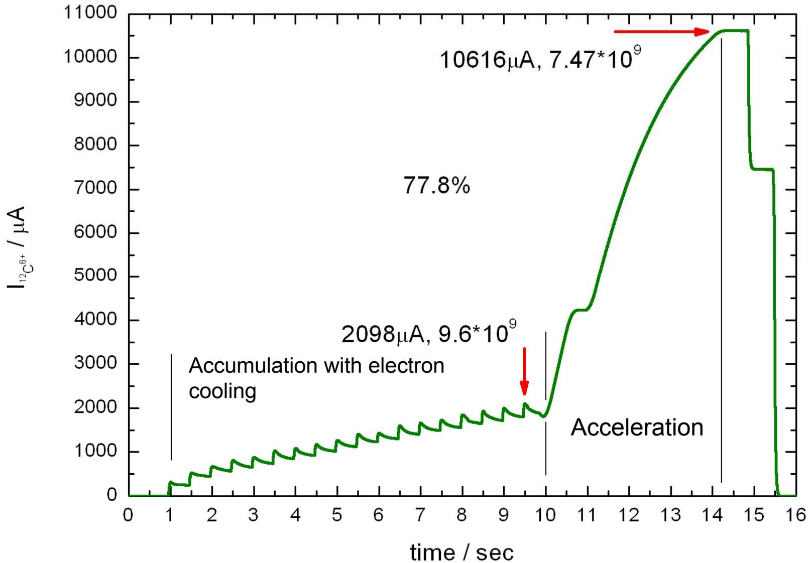
Cycle of accumulation and acceleration Carbon beam
