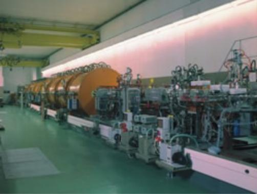
UNILAC—a 120-meter long linear accelerator—accelerates the ions to 20 percent of the speed of light. 11 MeV/u
