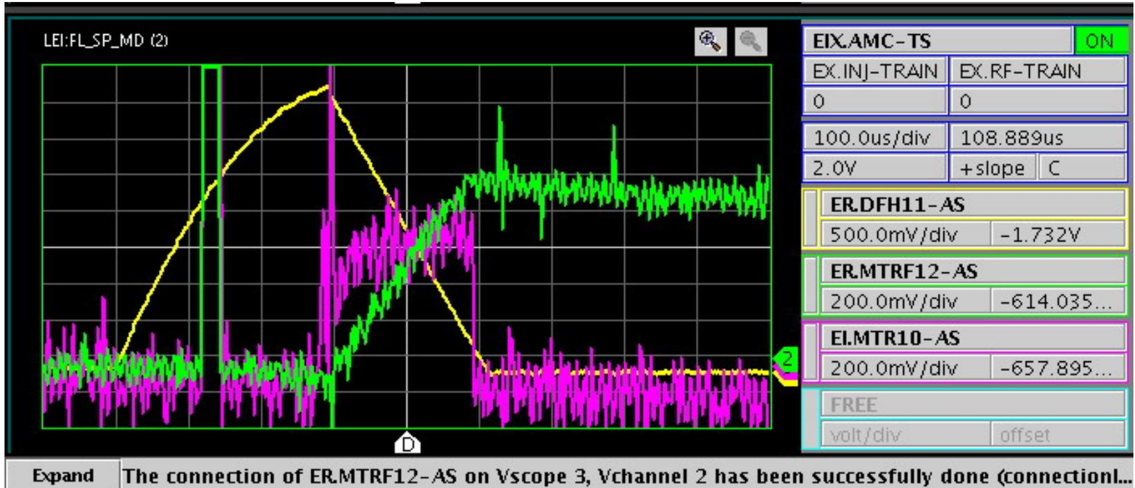
Yellow- bump magnet current, magneto- ion injector, green- ion beam accumulation at LEIR ring  $200 \cdot 10^{-6}$  s linear slope increasing storage ion current.
