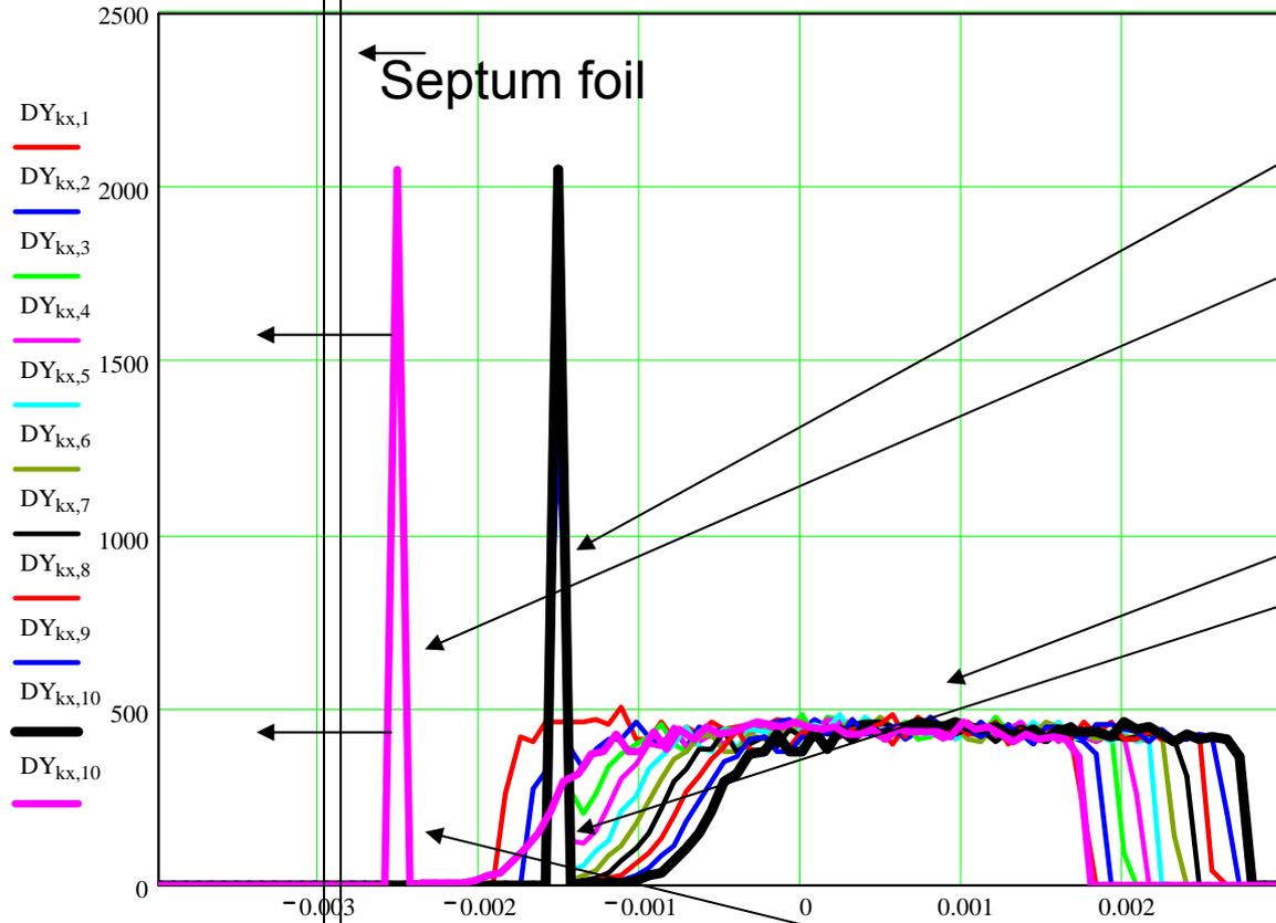
Electron cooler energy optimized for cooling to  $dp/p = -1.5 \cdot 10^{-3}$
