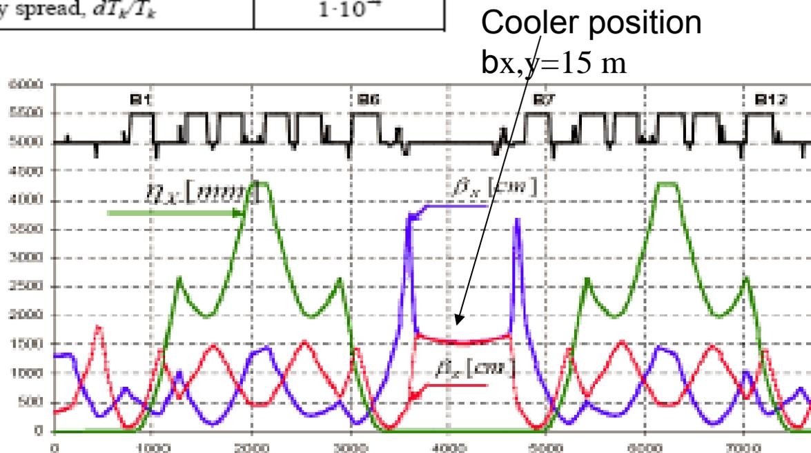
Figure 1: Synchrotron optical functions
