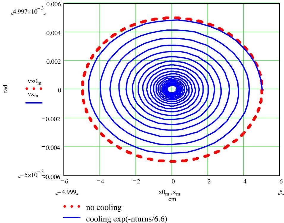
Cooling shrinks ion beam at intensive core with small radius and open phase space for new injection additional injection.
