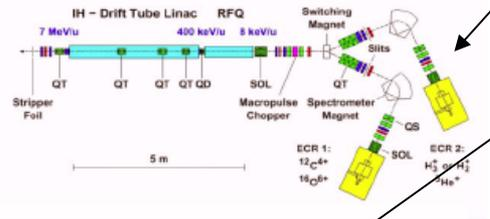
Figure 4: Layout of the injector-linac.
