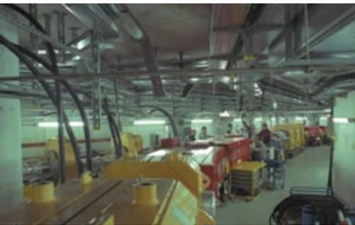
In the heavy-ion synchrotron SIS, the ion beam is further accelerated up to 90 percent of the speed of light in the course of several hundred thousand revolutions. Energy 2000 MeV/u Diameter of ring ~80 m
