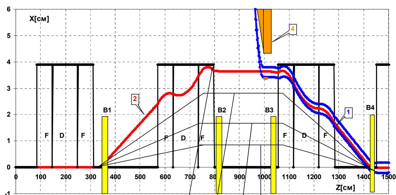
Injection multi turns with filling all available booster aperture.
