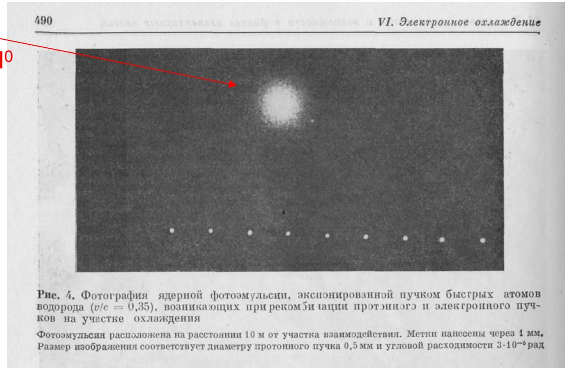
Distance from cooler to detector 10 m, energy of proton beam 65 MeV,
