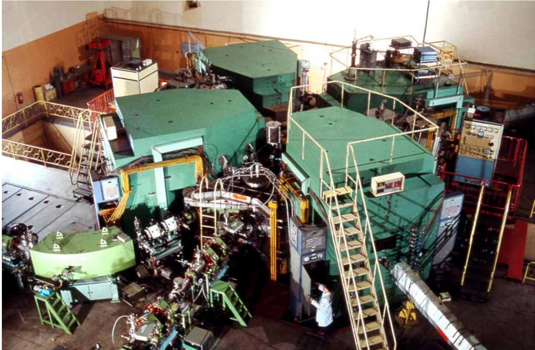
$K \sim 450$ ,  $R \sim 3.2$  m,  $E \sim 100$  MeV/u(C), 10 MeV/u(U),  $\epsilon \sim 10 \pi$  mm mrad,  $\Delta P/P \sim \pm 0.15\%$
