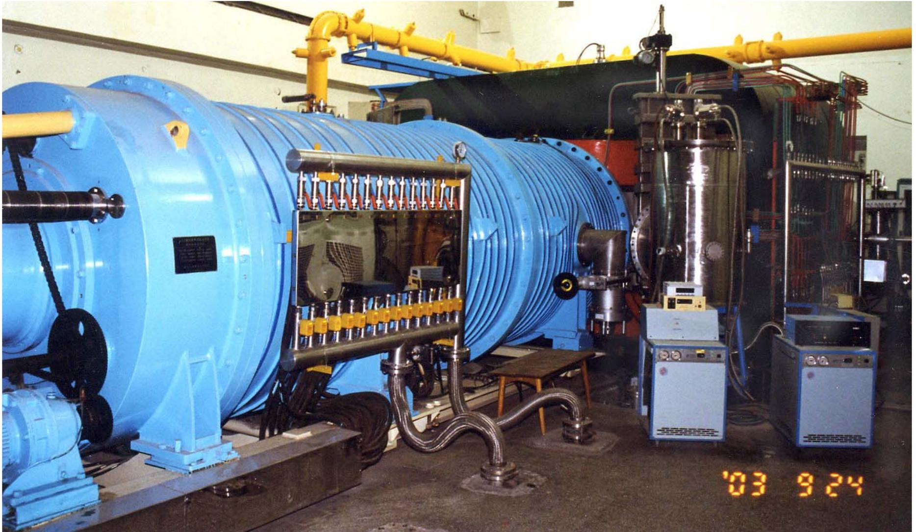
$K \sim 69$ ,  $R \sim 0.75$  m,  $E \sim 10$  MeV/u(C), 1 MeV/u(U),  $\epsilon \sim 20 \pi$  mm mrad,  $\Delta P/P \sim \pm 0.5\%$
