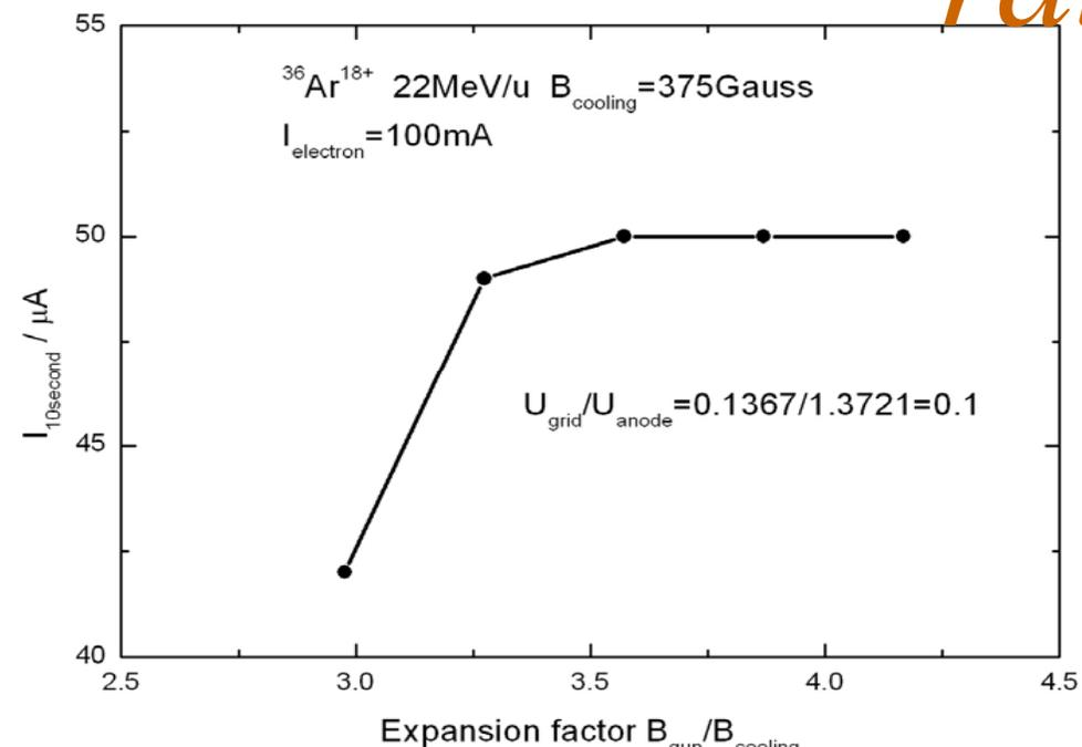
Expansion factor  $B_{\text{gun}}/B_{\text{cooling}}$
