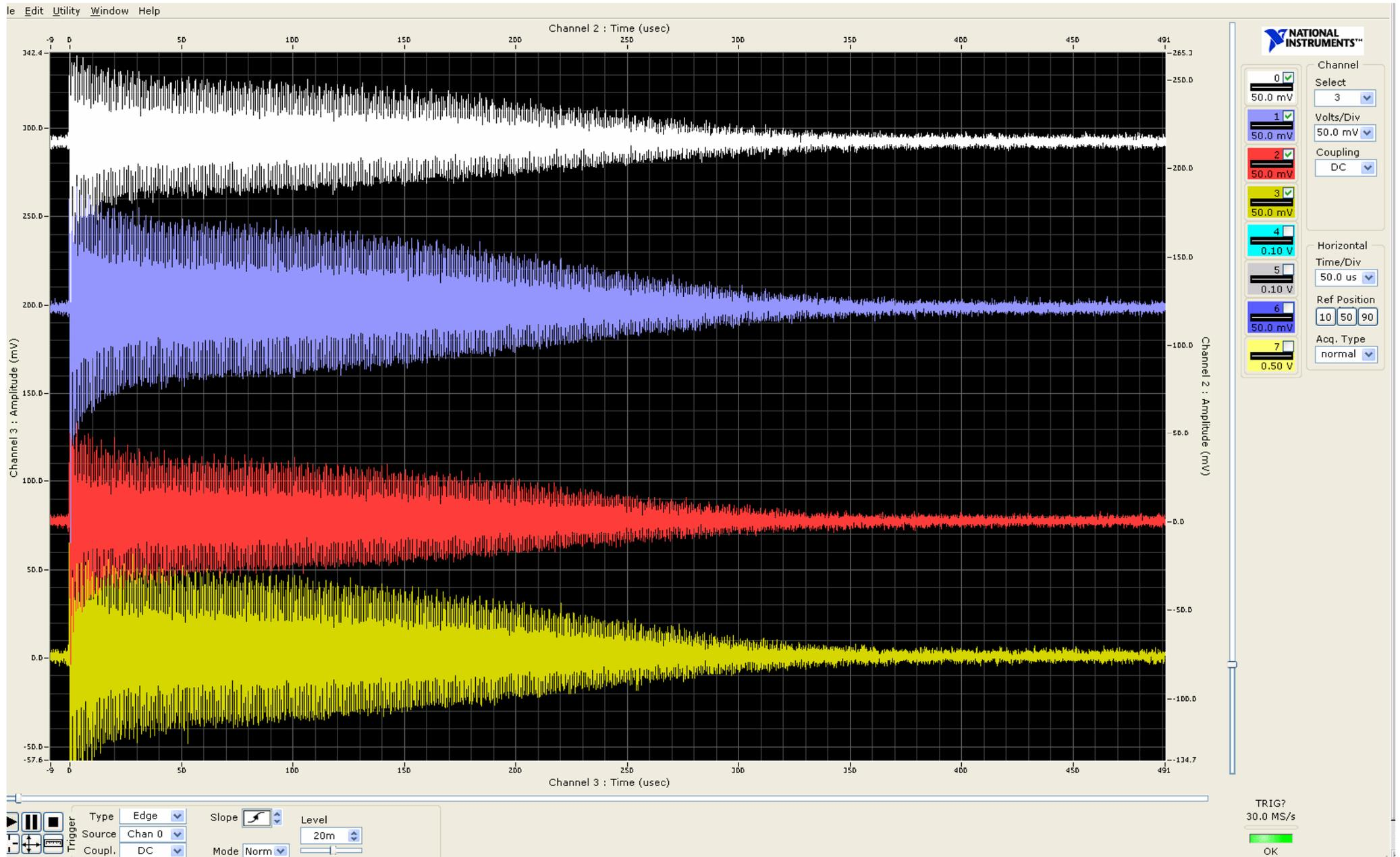
Turn by Turn Signals of Single Particle
