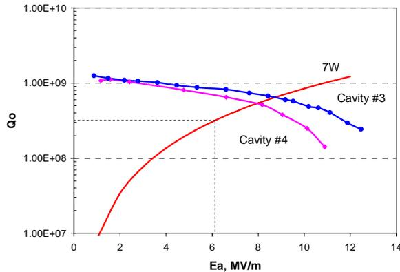
Fig.3. RF characterization results for prototype cavities
