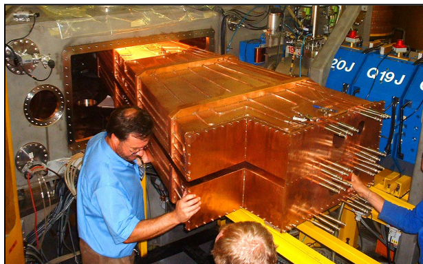
Figure 5: The flat-topping resonator of the SSC.
