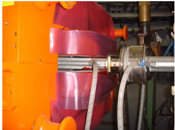
Fig. 1. Photo of radiation sensitivity film placed on the bending magnet inside the ring.
