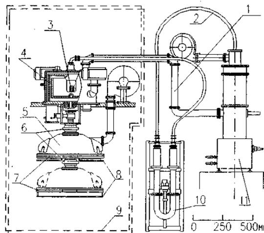
Figure 1: ILU-8 accelerator in local radiation shield.
