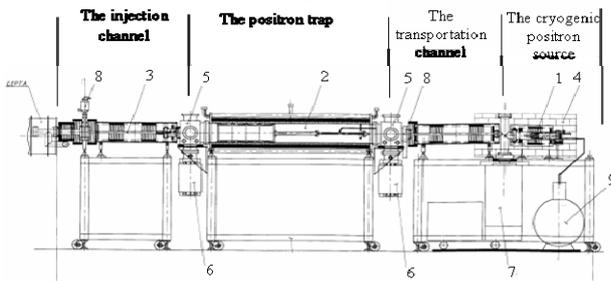
Figure 1: Positron injector. 1 - positron source  $^{22}\text{Na}$ , 2 - positron trap, 3 - vacuum insulator, 4 - radioactive protection shield, 5 - vacuum chamber for pumping out and diagnostic tools, 6 - ion pump, 7 - turbo pump 8 - the vacuum valve, 9 - LHe reservoir.
