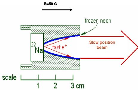
Figure 3: Slow positron getting principle.
