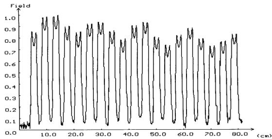
**Fig.6 BTW structure electrical field distribution**
