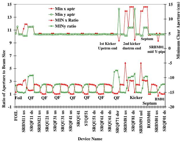
Figure 2. Minimum physical clear apertures and minimum aperture to beam ratios for the present Proton Storage Ring.
