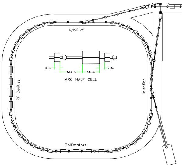
Figure 1: Accumulator ring layout.
