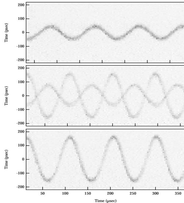
Figure 3: Images of the longitudinal profile (in psec) vs.time using the streak camera in dual scan mode: top)  $f_m$  below frequency of notch in BTF; middle)  $f_m$  at frequency of notch; bottom)  $f_m$  above notch frequency.
