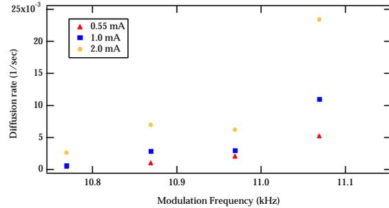
Figure 7: Diffusion rates as a function of modulation frequency for 3 different bunch currents.
