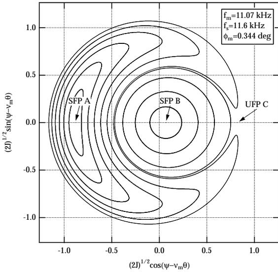
Figure 4: Phase space diagram in a frame rotating at the modulation frequency. The two stable fixed points are shown.
