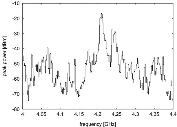
**Figure 2:** Typical beam excited dipole mode spectrum measured at a single structure (20-3c).
