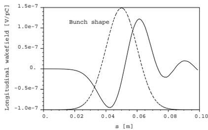
Figure 3: Longitudinal wakefield of the LER arc vacuum chamber.  $\sigma_z = 1$  cm.
