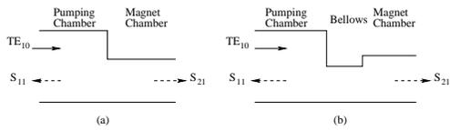
Figure 5: Schematics for S-parameter calculations at (a) the pumping-to-magnet chamber transition; (b) the bellows transition.
