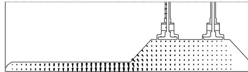
Figure 6: Electric field pattern at the BPM for the TE<sub>10</sub> mode propagating in the magnet chamber.
