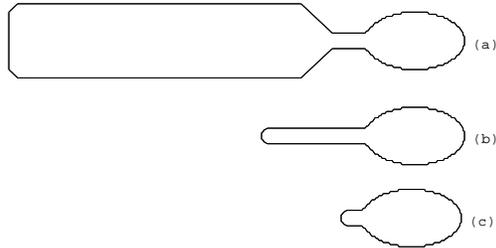
Figure 2: Cross sections of (a) the pumping chamber; (b) the magnet chamber; and (c) the bellows chamber.
