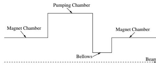
Figure 1: Schematic layout of LER arc vacuum chamber.
