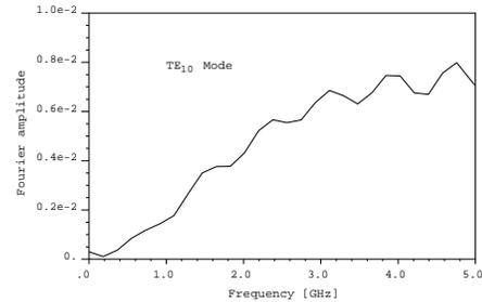
Figure 4: Fourier transform of the  $TE_{10}$  mode amplitude generated by the BPM.
