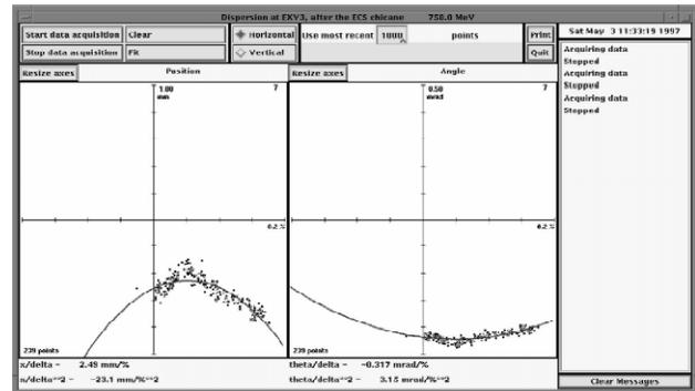
Fig. 4 Measured horizontal dispersions after the ECS chicane with the sextupole ESX1 set to  $+3.00 \text{ A}$
