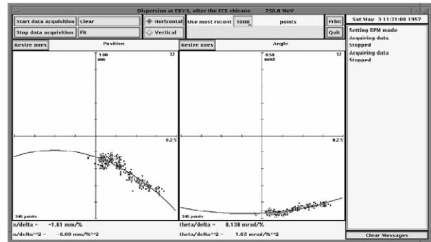
Fig. 3 Measured horizontal dispersion after the ECS chicane with the sextupole ESX1 set to  $+0.155\text{A}$
