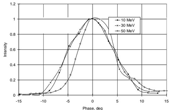
Fig. 3 Typical longitudinal profiles for normal mode of Linac-III operation
