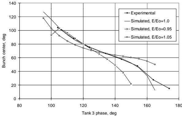
Fig. 6 Experimental and theoretical behavior of the bunch centers at the exit of the Tank 3.
