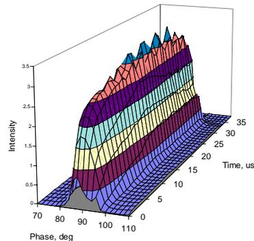
Fig. 4 Bunch shape evolution along the beam pulse at the exit of the Tank 1.
