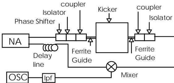
Figure 1: Phase Bridge Measurement Setup
