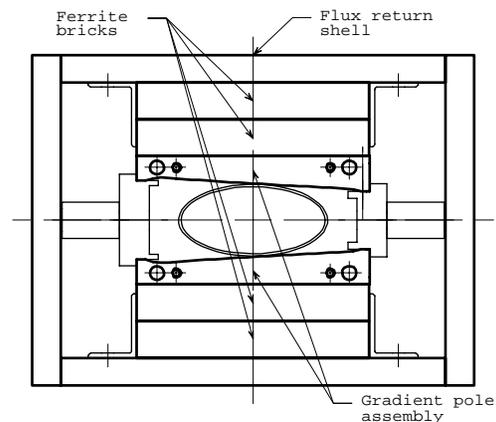
Figure 1: Recycler gradient cross section
