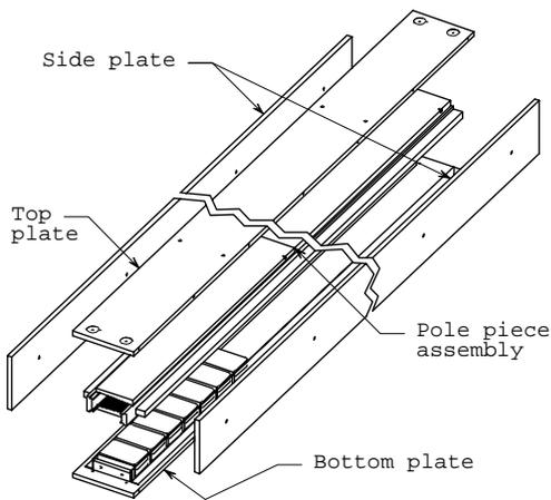
Figure 2: Recycler gradient exploded view
