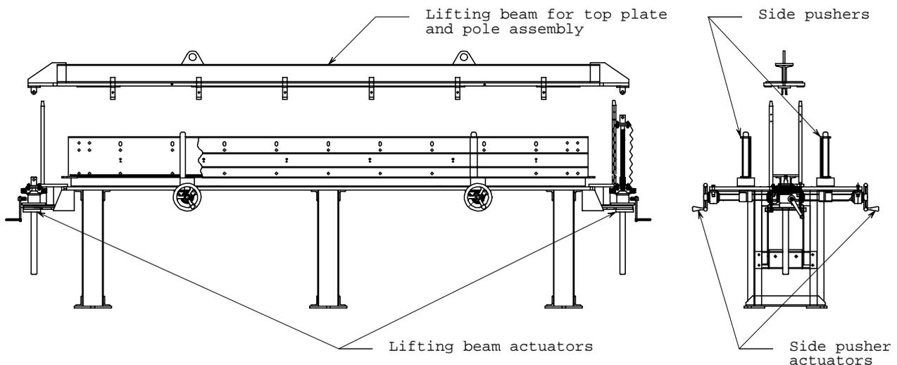
Figure 3: Permanent magnet assembly tooling
