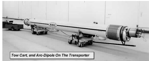
**Figure 2: Arc Dipole On Transporter**
