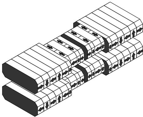
Figure 2: Phasing section for Pure Permanent Magnet. The distance between the magnet array is 6 mm (3 mm) for a period of 42 mm (20 mm).
