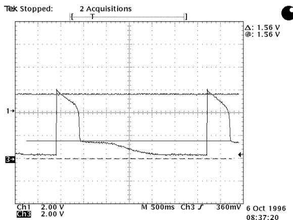
Fig. 4 The time-change of the stored beam-intensity in the injection current of  $780\mu\text{A}$  when the rf is turned off. The working point is (3.685,3.176). The vertical scale corresponds to  $6.0 \times 10^{10}$  ppp/div and the horizontal scale is 500ms/div.
