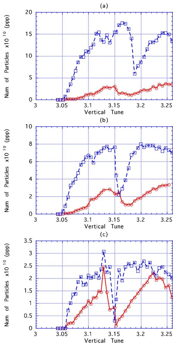
Fig. 3 The dependence of the stored intensity after 0.1s of the injection on the vertical tune. The injection peak current of (a)  $780\mu\text{A}$ , (b)  $300\mu\text{A}$ , and (c)  $100\mu\text{A}$ . The broken and the solid lines indicate the coasting beam (rf-off) and the bunched (rf-on) beam case, respectively.
