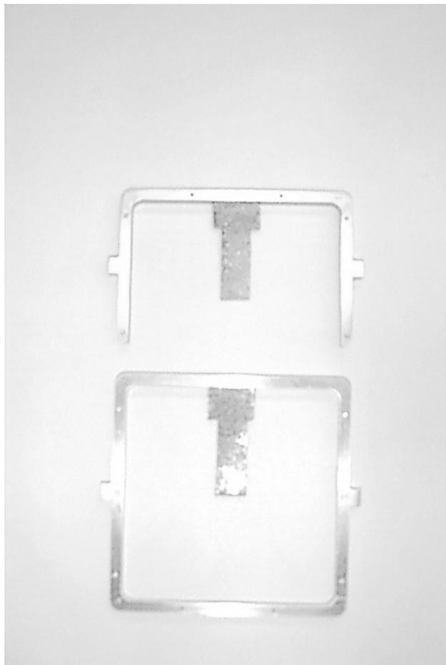
Fig. 1. Aluminum frames with carbon foil and fibers.
