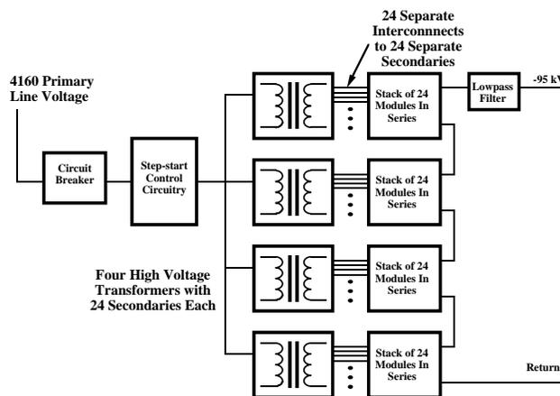
Figure 4. Solid state power supply topology.
