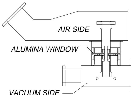
Figure 5. 350 MHz RF coaxial window.
