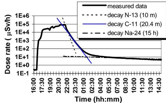
Fig. 5 Dose rate in the SINQ cooling plant room from short lived isotopes in the cooling water during and after the high current test of Dec. 4, 1996.
