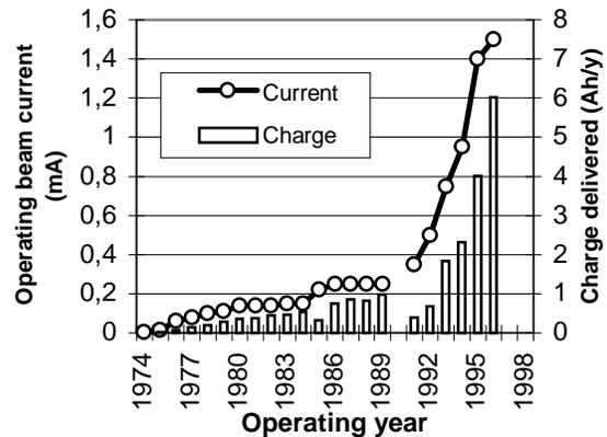
Fig. 1. Evolution of the beam current of the PSI accelerators from 1974 to 1995. The bars show the total beam charge delivered per year. In 1990 one of the two target stations was completely rebuilt and the ring upgrade program was started.
