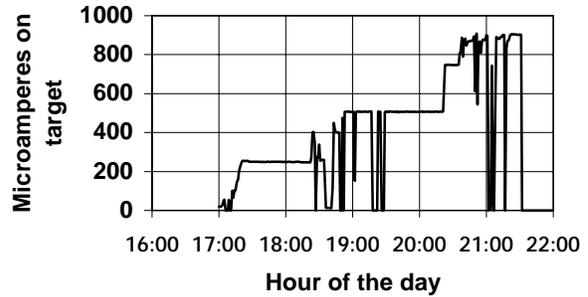
Fig. 4 High current beam test of the SINQ target on Dec.4,1996. The beam trips were mainly caused by low levels set in loss monitors. At 21:35h the charge limit of 2 mAh was reached
