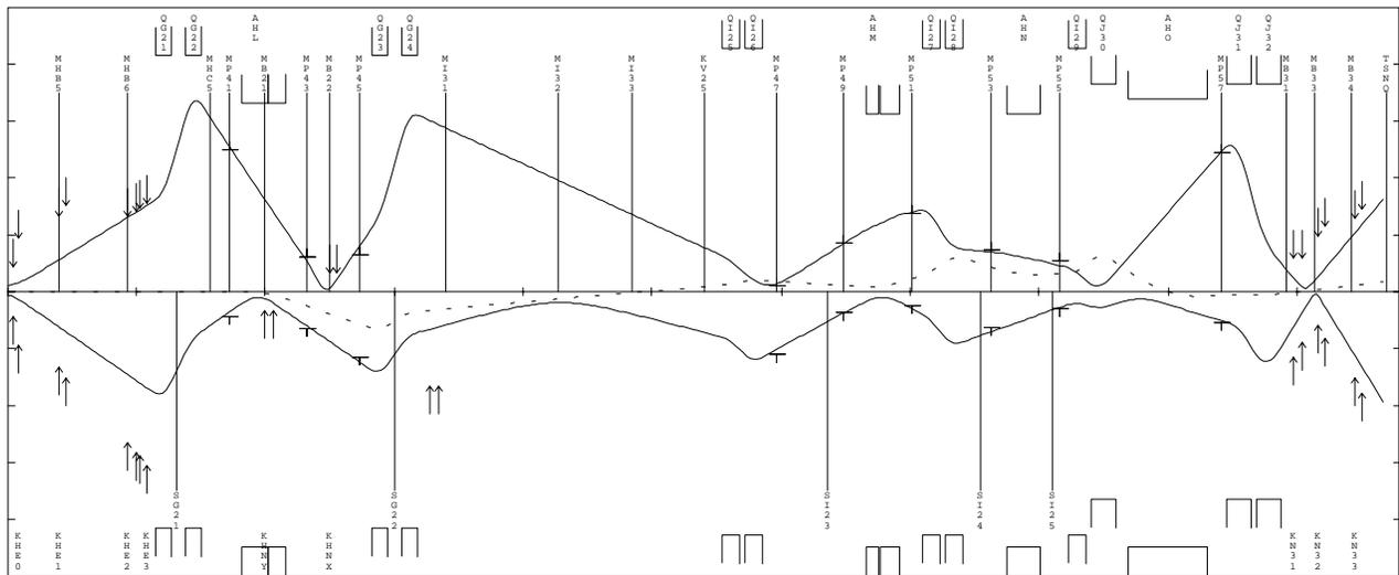
Fig 3: Envelope fit for the 900  $\mu$ A beam during the commissioning of the new proton beam line.  $\Uparrow$  and  $\Downarrow$  represent measured beam widths. The lower and upper half-frames show data for the vertical (bending) plane and the horizontal plane respectively. Computations were done with the code TRANSPORT. Full scale in both direction is 15 cm. The dotted line shows the assumed 1% dispersion trajectory.  $\uparrow$ ,  $\downarrow$  symbolize slits and collimators.
