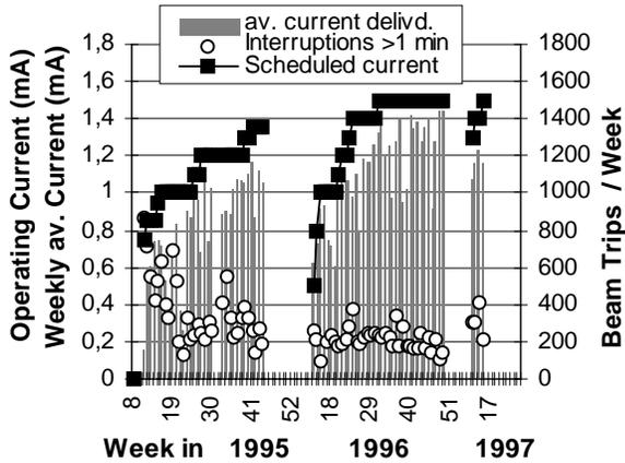
Fig. 2: 590 MeV operation of the PSI accelerators since 1995.
