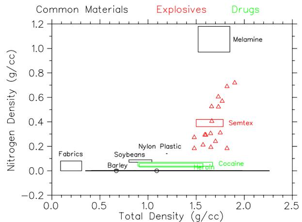
Figure 1: Explosives have a unique signature compared to common materials when nitrogen density is plotted against total density
