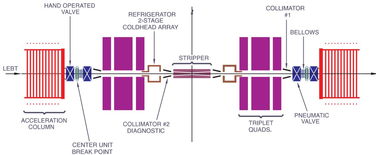
Figure 4: Schematic layout of the terminal vacuum system
