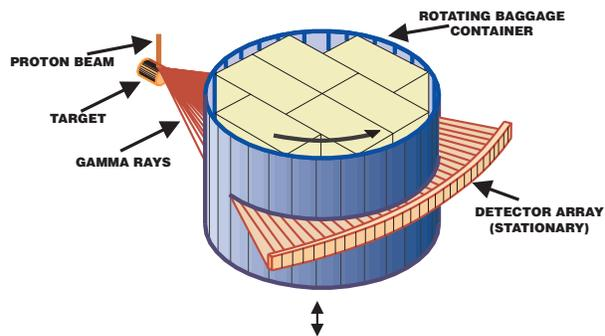
Figure 2: CDS detector and inspection geometry
