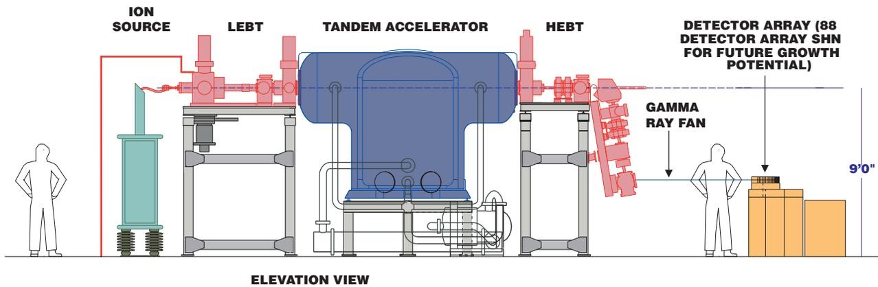
Figure 3: Side elevation of the CDS proof-of-principle device
