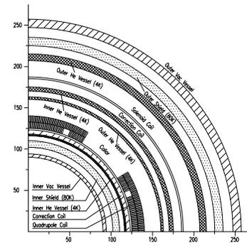
Figure 3: Cryostat cross section at the middle of Q2.
