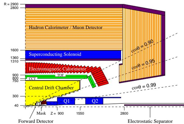
Figure 1: Schematic layout of the detector facility and IR accelerator components.
