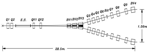
Figure 2: Magnet layout in the interaction region.
